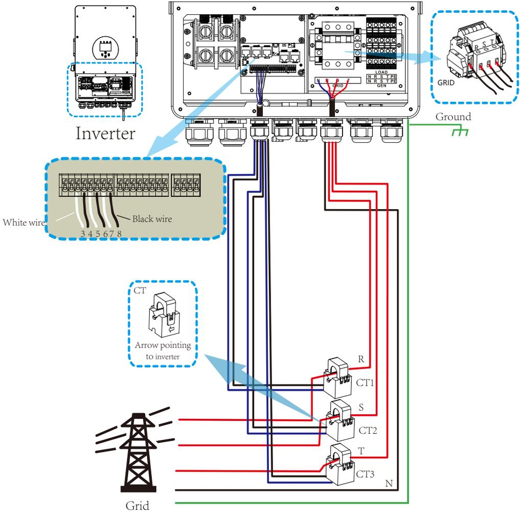
**\*Note:** when the reading of the load power on the LCD is not correct, please reverse the CT arrow.
