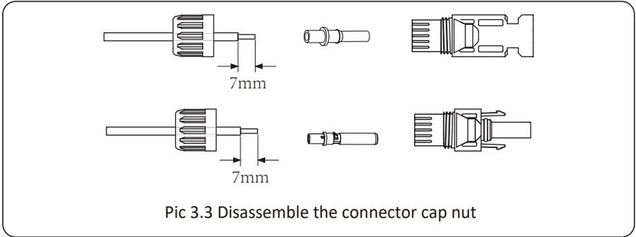
Pic 3.3 Disassemble the connector cap nut
