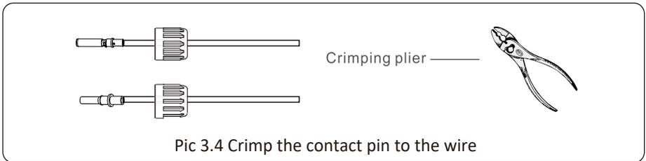
Pic 3.4 Crimp the contact pin to the wire
